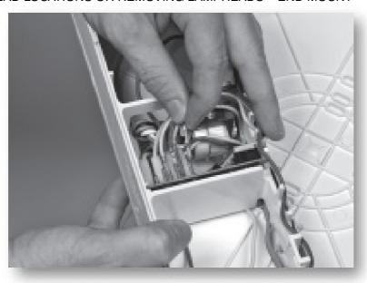
Disconnect lamp leads at the printed circuit board.
