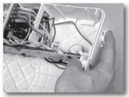
Press the fit hole plugs into the old lamp head hole location.
