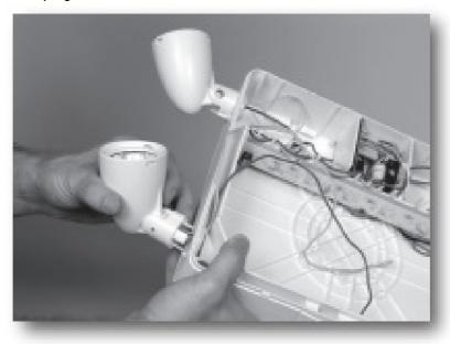
Route lamp leads through new hole location and press fit lamp head into a new location.
