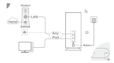
1. Connect the power adapter to your router, then connect the WAN port of the router to the LAN port of the optical/broadband modem or a wall-mounted network port using a network cable.
