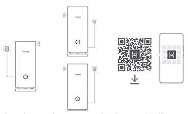
4. If the pack you purchased contains more than one router, the other router(s) will set up a network with the first configured router automatically after being connected to the power supply.
