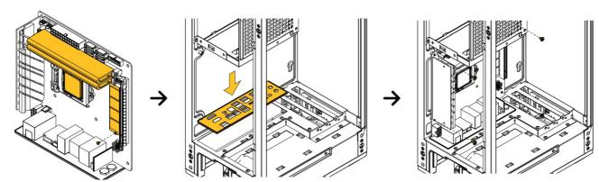
5. **Cable Manage Motherboard** – Complete as much cable management as possible before installing the CPU cooler.
