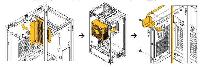
3. Remove GPU Cable Cover and Open Radiator Door
