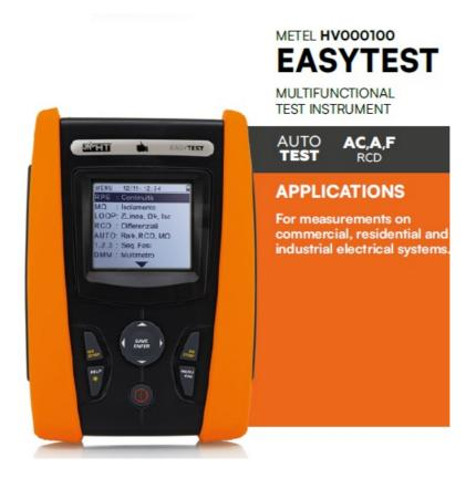
**AUTOMATIC test (Ra, RCD, Insulation)** in sequence, continuity of protective conductors with 200mA, Insulation resistance up to 1000V, polarity test, RCD testing type A, AC, F General and Selective up to 1A, line impedance and presumed short-circuit current measurement, testing of thermal-magnetic circuit breakers and fuses, Multimeter function to measure: Frequency, VL-N, VL-PE, VN-PE. Cyclic phase direction, voltage drop, internal memory and PC connection.
