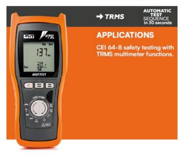
**AUTOMATIC sequence:** global earth resistance, tripping time of RCDs type A 30mA, AC up to 300mA, tripping current of RCDs type A and AC 30mA (Ramp test), 250V or 500VDC insulation resistance measurement, continuity of protective conductors with 200mA, cyclic phase direction with 1 or 2 terminals, leakage current measure-ment with optional clamp HT96U\* Multimeter TRMS: AC/DC voltage, resistance and continuity, frequency.
