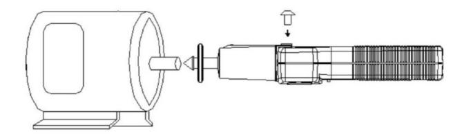
Fig. 3: attach of mechanical adaptor
