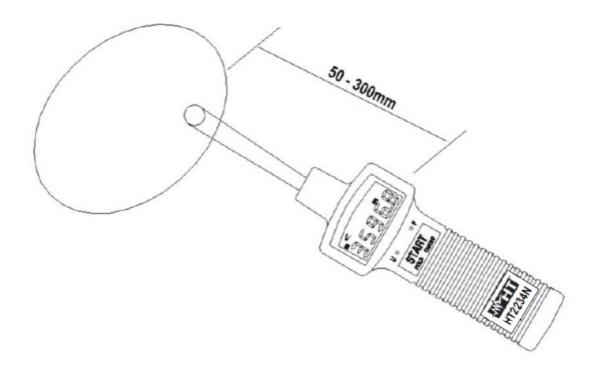
Fig. 2: speed measure without contact (RPM)
