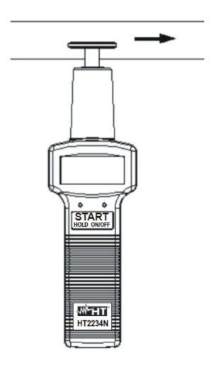
Fig. 4: speed measure on surfaces
