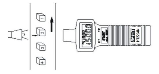
Fig. 5: events counter with external light source
