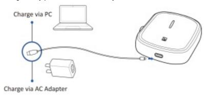
**Note:** The printer can be charged via a computer USB port or AC adapter. Please note that the AC adapter is not supplied.
