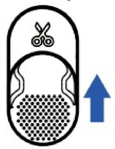
04 Push the cutter button to manually cut the paper.
