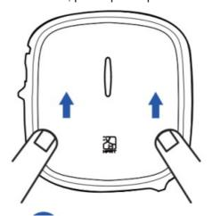
Load the paper as shown in the figure and make sure the thermosensitive layer faces up.
