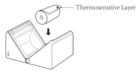
3. Move the paddle switch up and adjust the paper limiter according to the width of the paper roll. After adjustment, press down the paddle switch and lock the paper limiter
