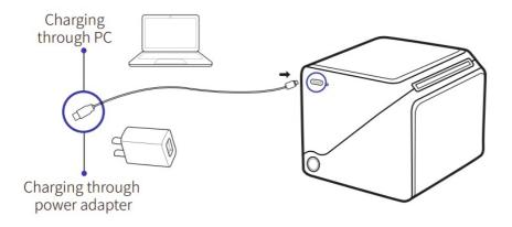
**Note**: You can use a power adapter or computer USB for power supply, and the adapter is not included when shipping. If consumers use a power adapter for charging, they should purchase and use a power adapter that has obtained CCC certification and meets the standard requirements
