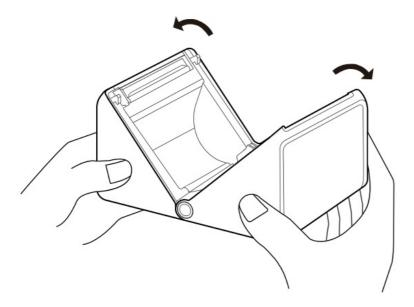
2. As shown in the following figure, install the paper roll with the thermal side facing outward.
