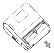
3. Battery Pack Installation reference to the positive and negative electrodes inside the battery bin identification corresponding to the battery, positive and negative electrodes installed in place;
