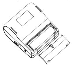
4. When installing the battery cover, two guiding ribs at the front end of the battery cover are inserted into the guiding groove of the cover Push the battery cover forward into place to complete the installation.
