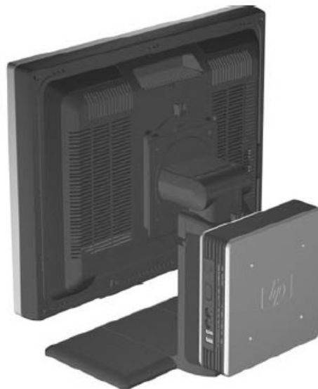
Figure 5-6 Thin client mounted on the back of monitor stand
