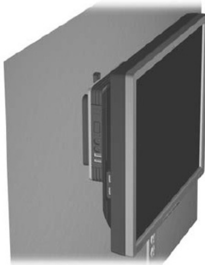
Figure 5-5 Thin client mounted with a flat panel on the wall
