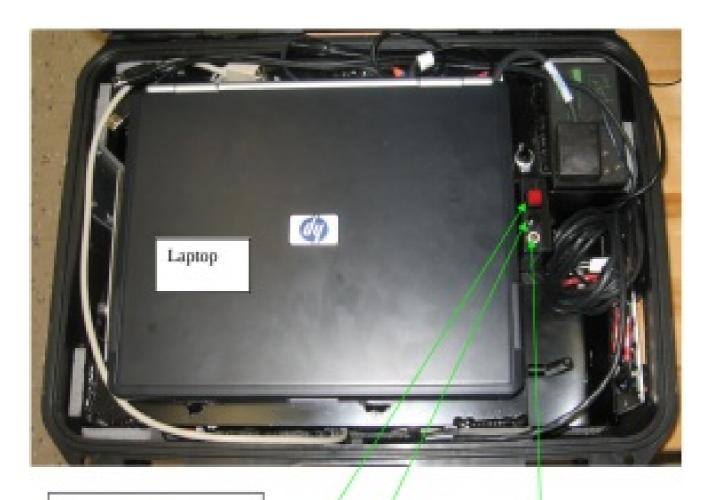
Switch to control power to the Nexus Hawk Router and the fan
