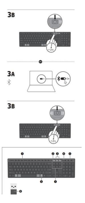
Connect the keyboard to one computer using the receiver and up to two computers via Bluetooth®. To program the keyboard keys or set up your keyboard and mouse to easily switch between computers, use the software. If the software does not download automatically, on your computer, open Microsoft Store. Search for HP Accessory Center, and then download the app.
