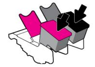
Open carriage latches and insert cartridges.
