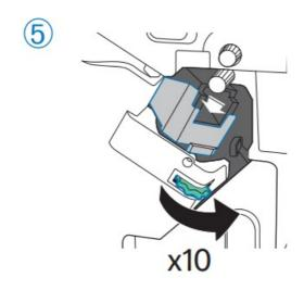
Hold the green wheel while installing the staple cartridge.
