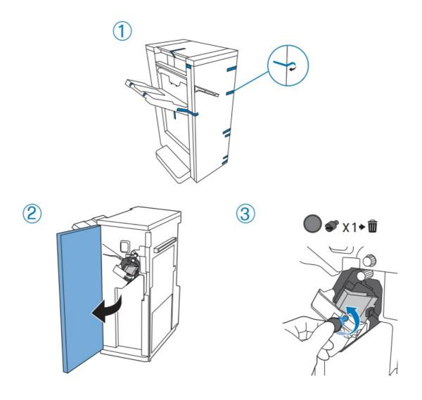
Rotate the green Wheel clockwise 10 times to move the staple unit to the installation position.
