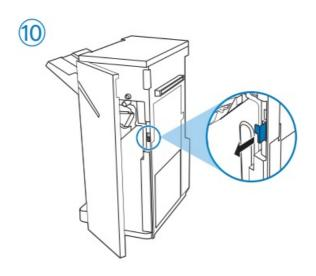
Firmly push the Finisher and Printer together until the locking mechanism clicks into place at all three marked locations.
