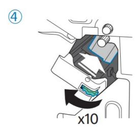
Once the cartridge slot is visible, rotate the green wheel counter-clockwise 10 times.
