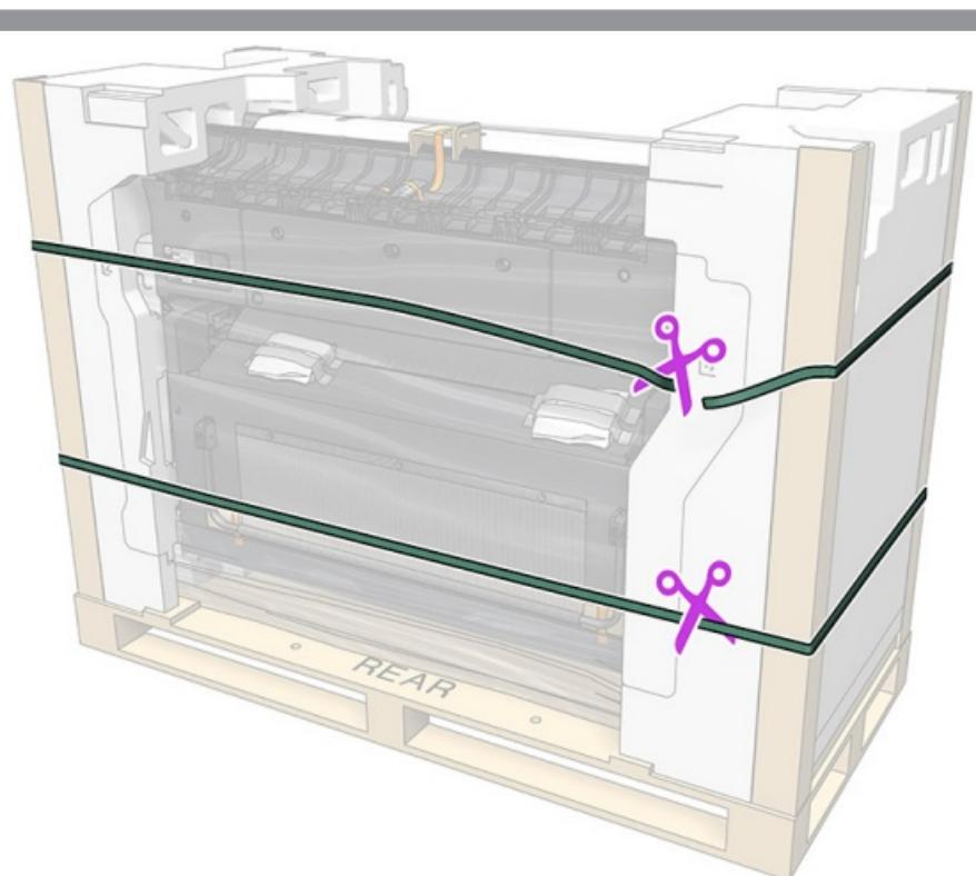
Cut and remove the horizontal plastic-straps.
