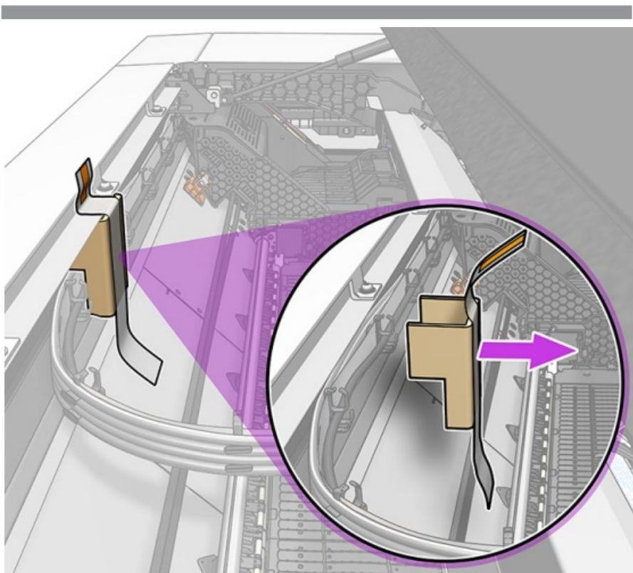
Remove tape and cardboard packaging that holds the SRK in place within the print zone. Pull away from the SRK at 90-degree angle (as pictured).
