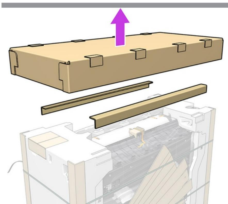
Remove the top carton-cover, then remove the wooden bars from inside of the box.
