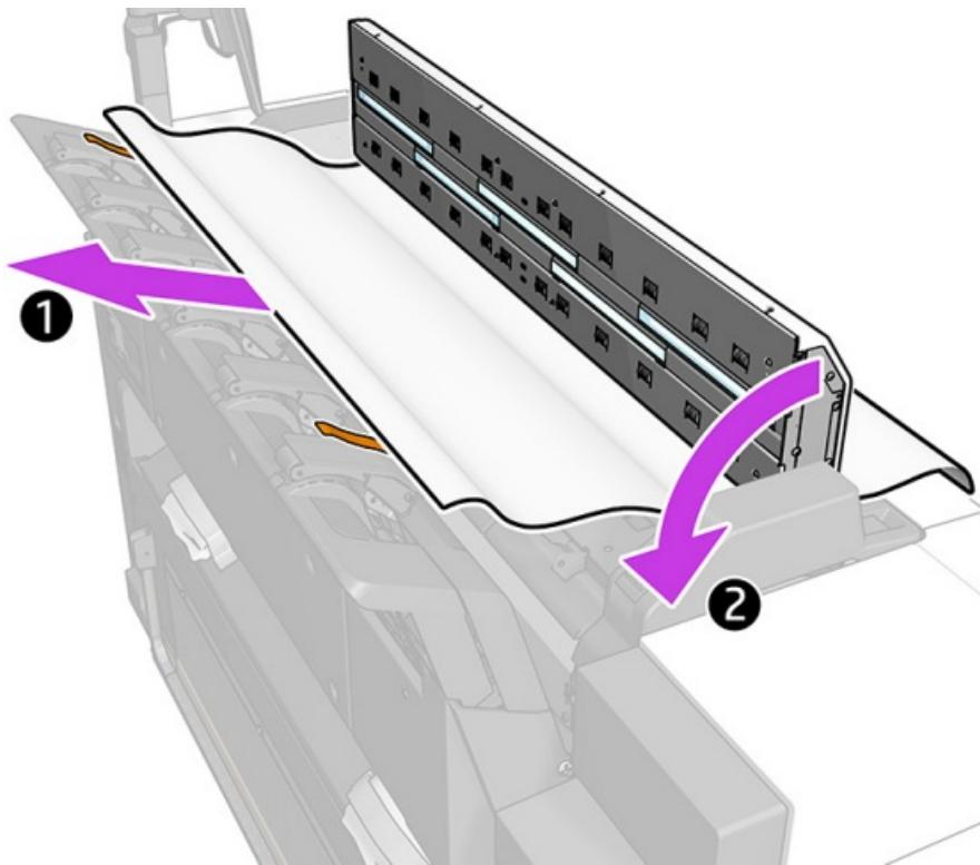
Remove the protective foam (1) and close the scanner (2).
