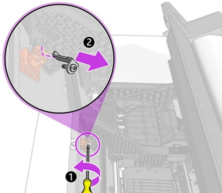
Remove the T15 screw and metal piece from the carriage.
