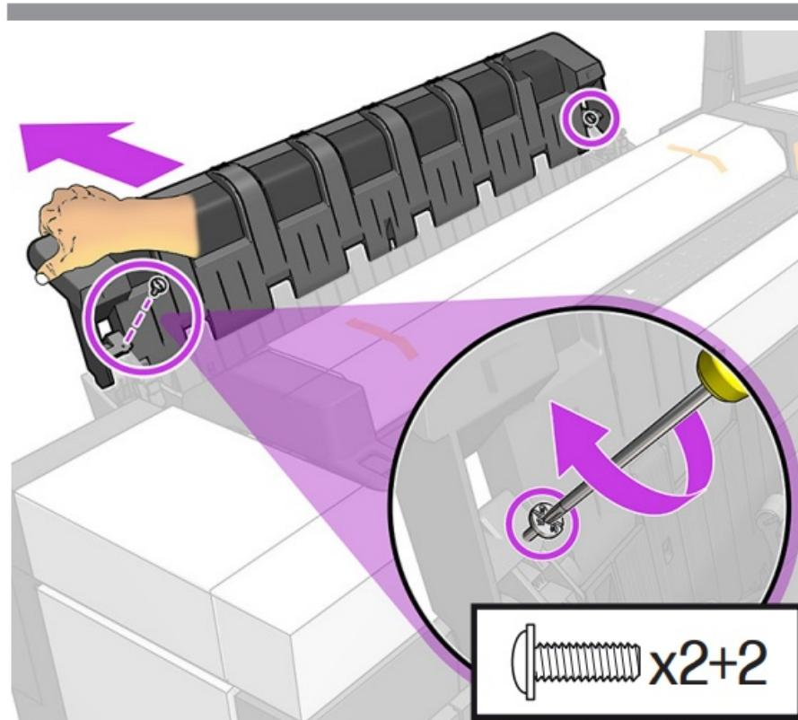
Pull the stacker back and hold it (1), then fix it into position with two T25 screws, one each side (2).
