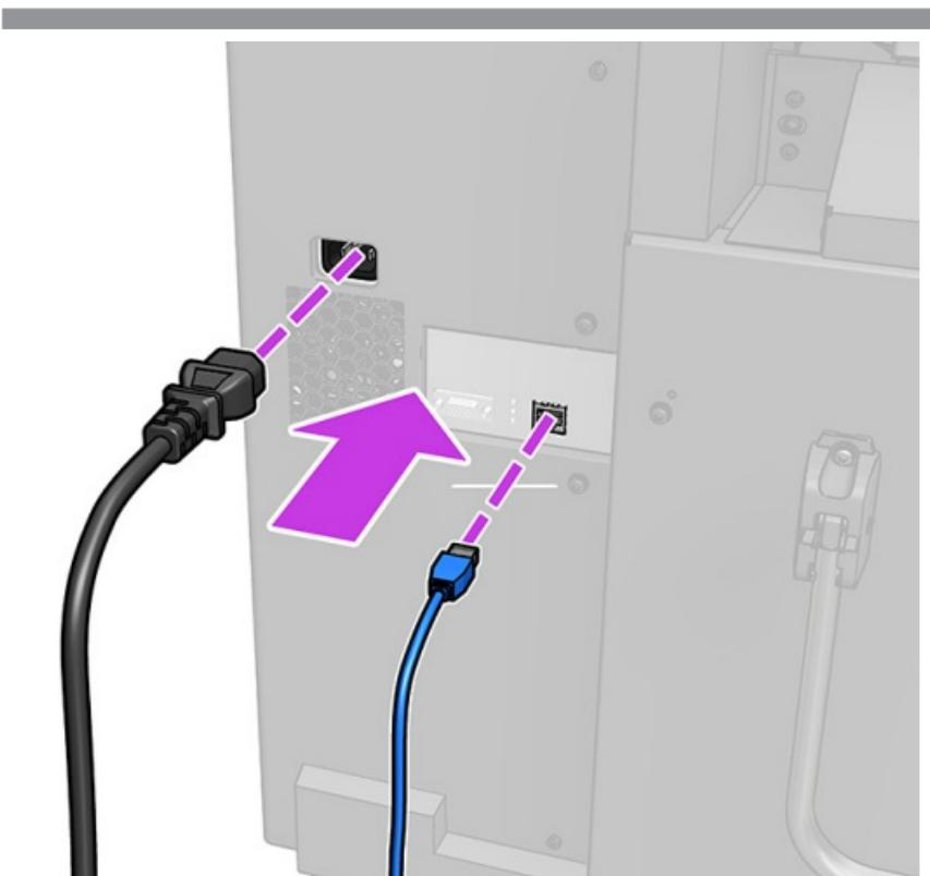
Connect the power cable and the LAN cable to the back of the printer.
