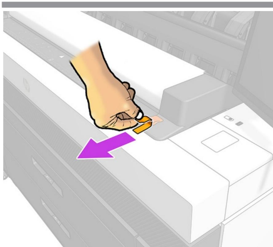
Remove the orange tape from the scanner locking key.
