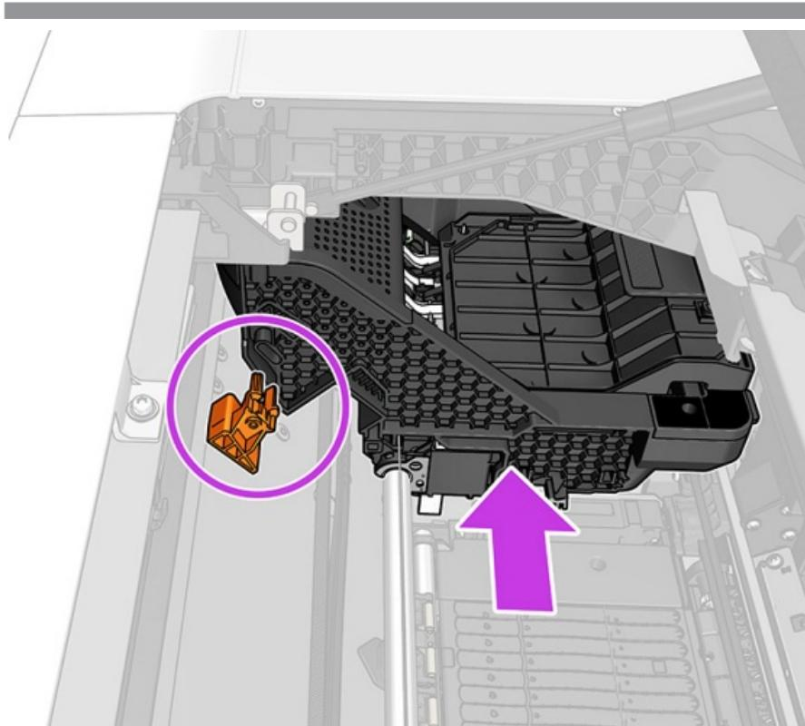
Push the carriage to the left to access the orange carriage-lock.
