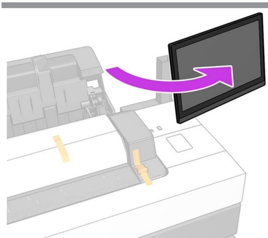
Rotate the control panel out of the way to create space.
