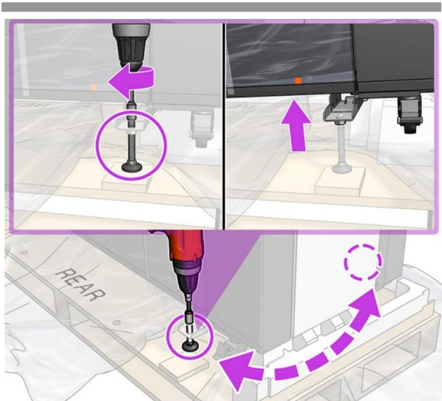
Little by little screw the bolts to elevate the printer until the endcaps are free from the pallet.
