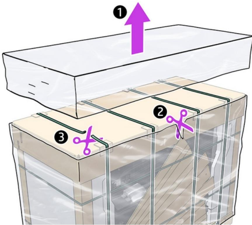
Remove the plastic covers from the top and around the printer (1+2). Cut and remove the vertical plastic-straps (3).
