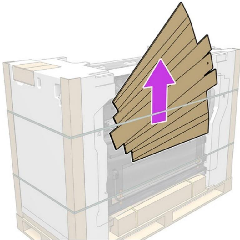
Remove the two unfolded cardboard ramps by lifting them upwards, and place them aside for later use.
