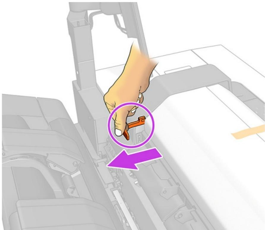
Remove the scanner locking pin by pulling it forward.
