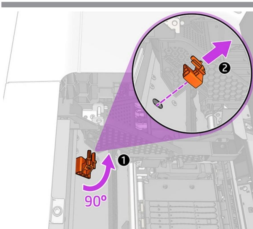
Remove the orange carriage lock by rotating it (1) and pulling it out (2). Close the scanner.
