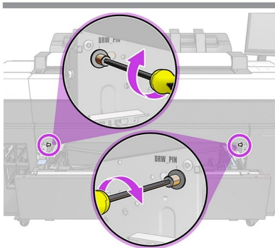
Insert the pins and screw (T25) them firmly into place.
