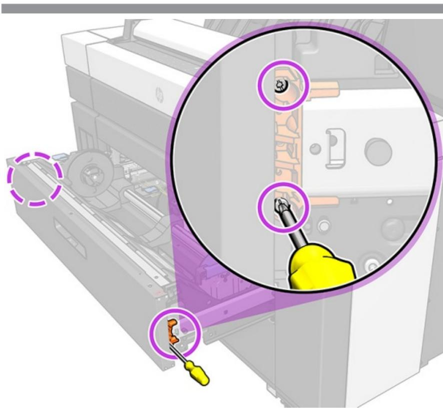
Remove the two T15 screws from each of the orange locks. There is one lock on each side of the drawer.
