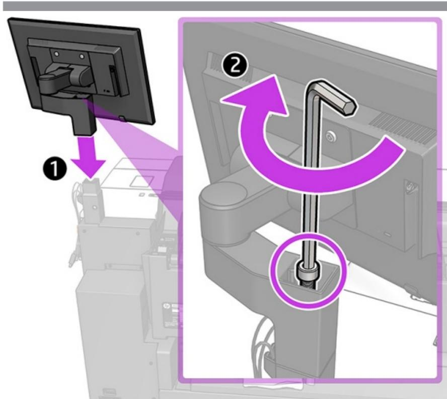
Insert the control-panel tube completely and tighten the screw.
