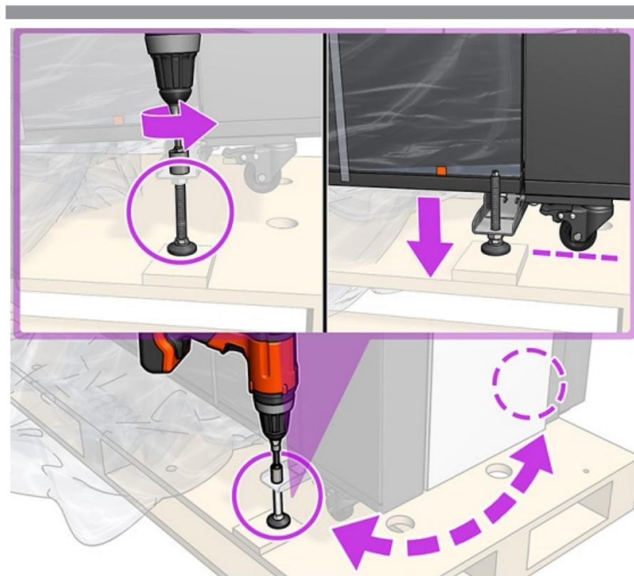
Lower the printer by reversing the step to lift it.
