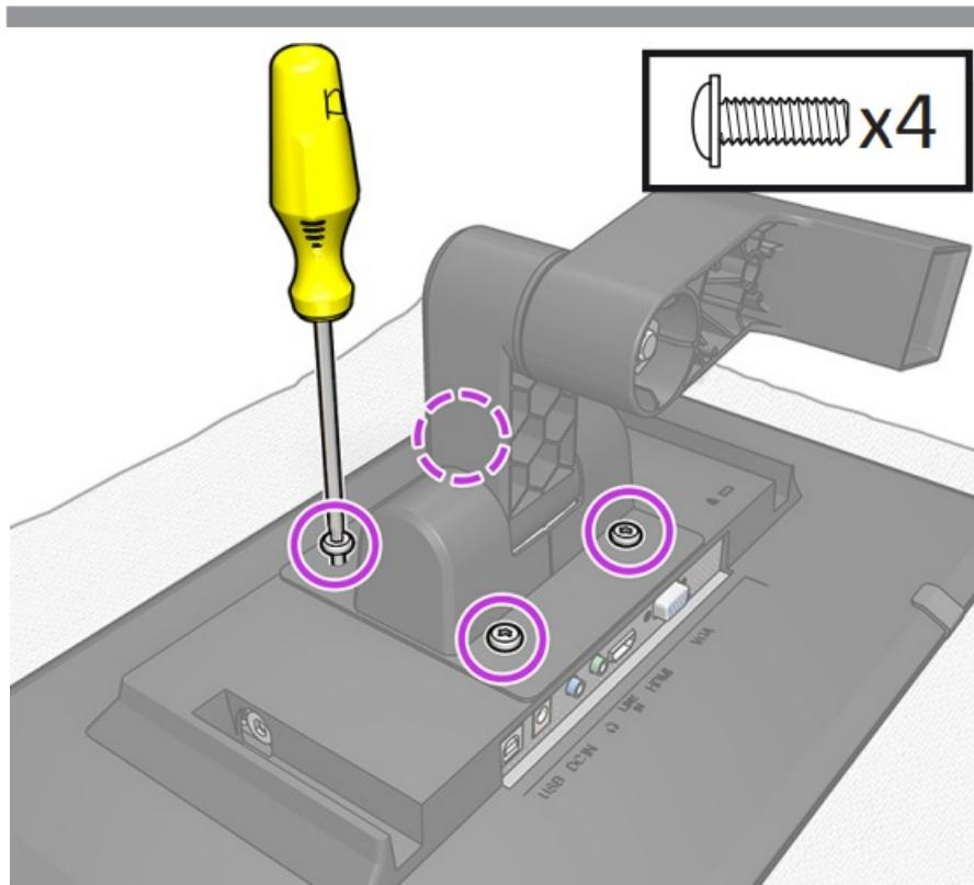
Attach the arm to the control panel using four T25 screws.
