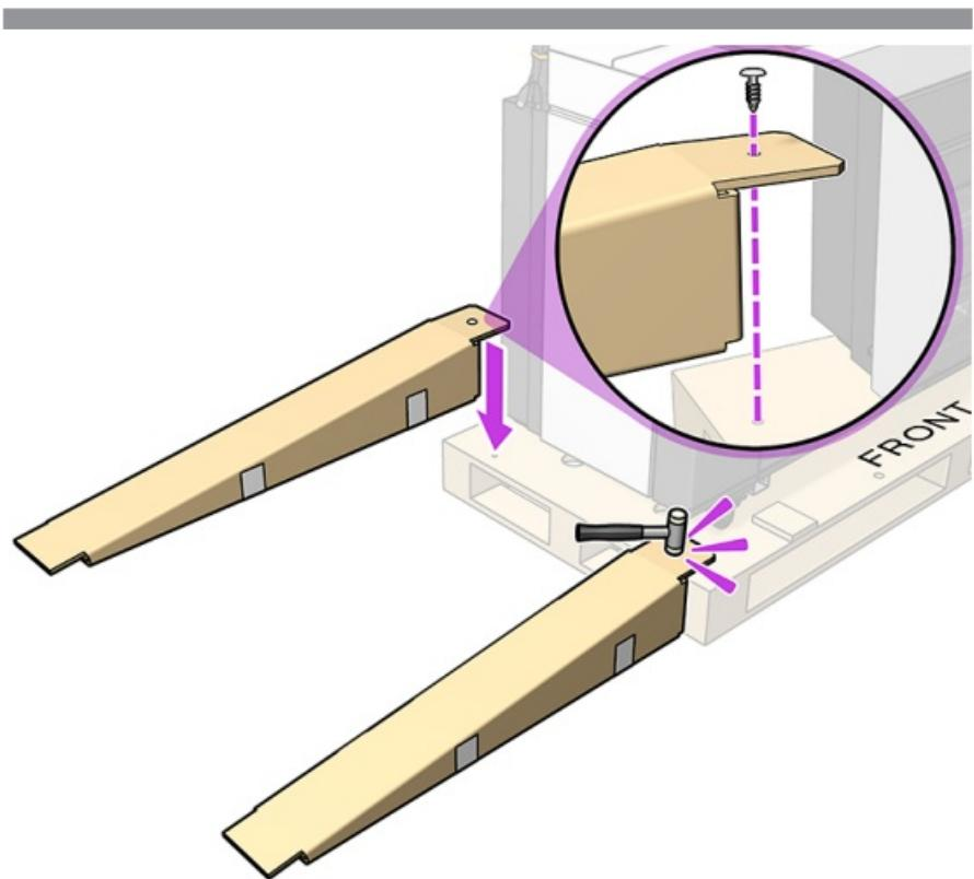
At the left side of the unit, use the white screws—located in the accessory box—to fix the ramps to the pallet.
