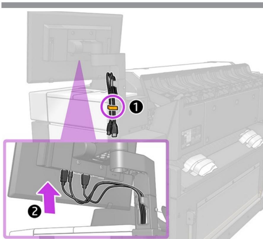
Remove the orange tapes and plastic bags, then route the cables through the control-panel support.
