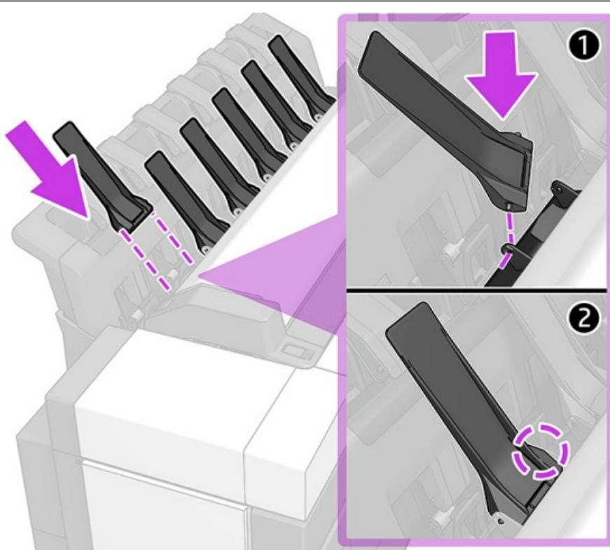
Insert the six deflectors; first insert one side (1) and then click the other side into place (2).
