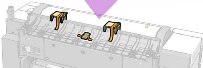
Remove the tray-holder locks and bag of stacker screws. Put the screws to one side for later.
