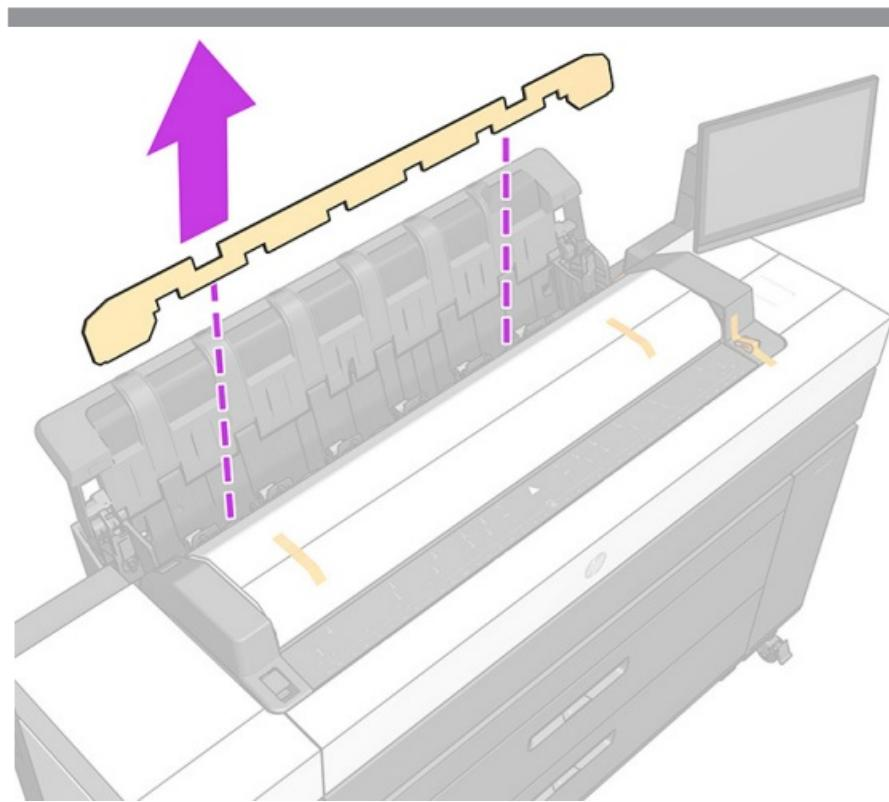
Carefully remove the carton from inside the stacker.
