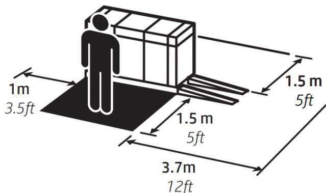
The size of the crate is 1718 mm x 766 mm x 1275 mm. The space required for assembly is 1.5 m (5 feet) at the front and back and 3.7 m (12 feet) at the side.
