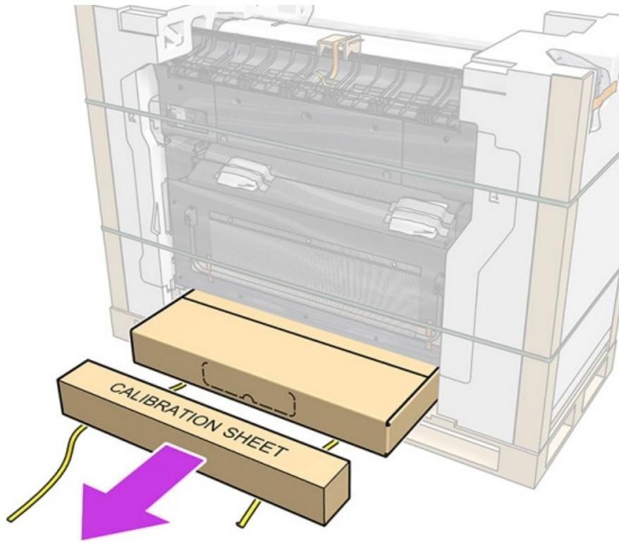
At the back of the unit, cut the yellow straps to free the two boxes of materials. Remove the boxes.
