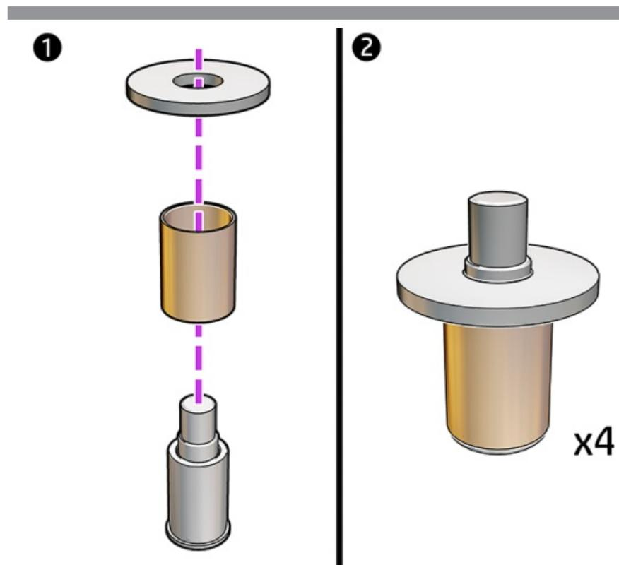
Assemble the four pins by adding a sleeve and washer to each one.
