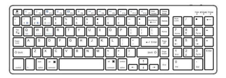
**Note:** All blue multi-function keys need to press "FN + blue function key" at the same time to achieve (For example, press "Fn" +" Q", the keyboard will switch to iOS system.)
