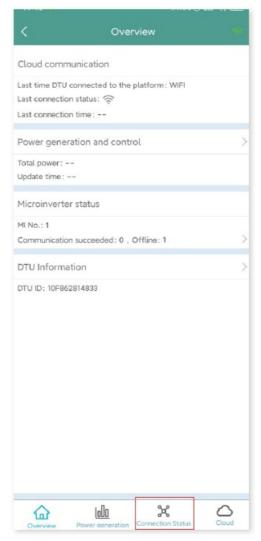
2. On this page, you can check the signal strength between the DTU and each microinverter. Tap the signal icon to enter the respective microinverter page (signal quality is constantly refreshed).
