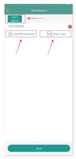
4. The search result of microinverters and microinverters added will be displayed in the list. Tap the button on the right if you want to delete it.
