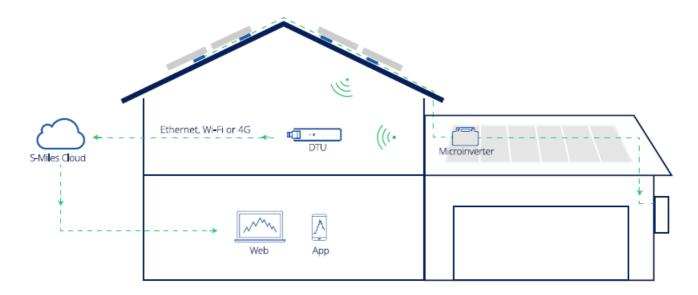
The complete Hoymiles PV microinverter system is composed of PV microinverter, Hoymiles gateway DTU and Hoymiles S-Miles Cloud.
