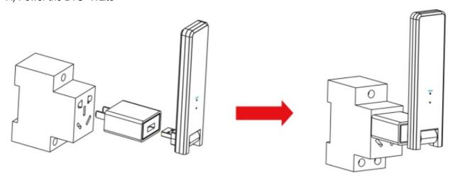
**Option 2:** Connect the DTU to the adapter and plug it into the Power Strip. Please make sure it is placed at least 0.5 meter above the ground and try to install the DTU 90 degrees vertical to the ground as much as possible.
