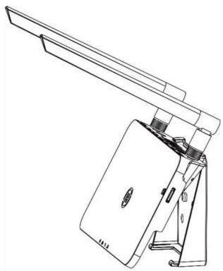
Match the bracket's lower buckle by gently press the lower side of the DTU-Pro until hear the Click.
