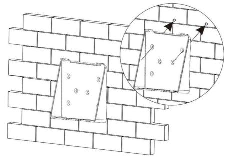
Match the bracket's upper buckle with DTU-Pro;
