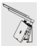
• Fix DTU-Pro-S to the bracket's lower buckle gently until you hear a click. Please make sure that the antennas are vertical to the wall.
