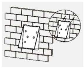
• Fix DTU-Pro-S to the bracket's upper buckle.
