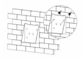
• Match the bracket's upper buckle with DTU-Pro;
