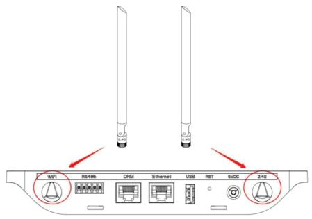
**Note** If the DTU installation location is inside the metal box or under the metal / concrete roof, extended 2.4G cable or 2.4G sucker antenna will be suggested, which can be purchased from Hoymiles or local electrical store (Please contact Hoymiles's Tech. support team for the detail type of the cable or antenna at <a href="mailto:support@hoymiles.com">support@hoymiles.com</a>.
