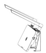
• Match the bracket's lower buckle by gently press the lower side of the DTU-Pro until hear the Click. Please make sure the antennas are vertical to the wall.
