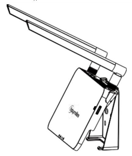
• Match the bracket's lower buckle by gently pressing the lower side of the DTU-Pro/DTU-Pro-Cuntil youhear a
