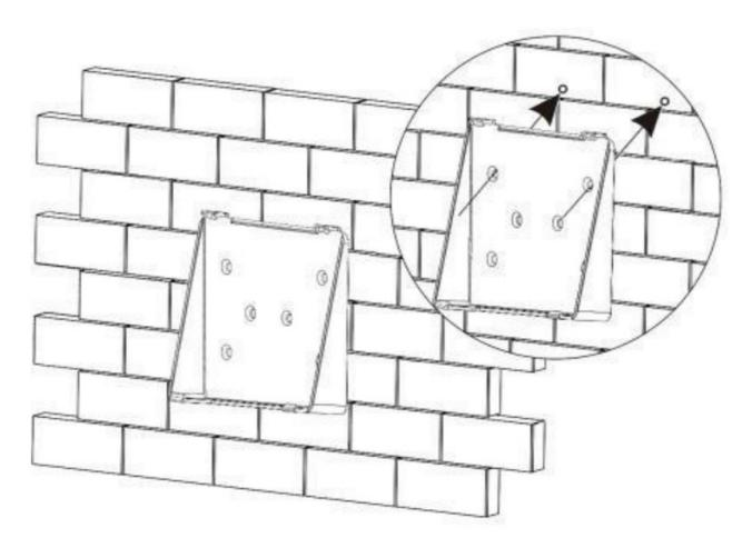
• Match the bracket's upper buckle with the DTU-Pro/DTU-Pro-C.
