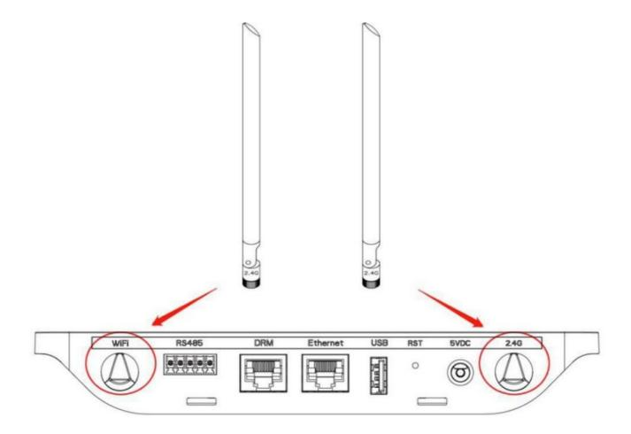
**Note:** If the DTU installation location is inside a metal box or under a metal/concrete roof, an extended2.4G cable or 2.4G suction antenna is suggested, which can be purchased from Hoymiles or a local electrical store (Contact Hoymiles Technical Service Center for the detailed type information of the cable or an tenna at <a href="mailto:support@hoymiles.com">support@hoymiles.com</a>).
