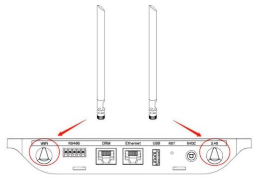
**Note:** If the DTU installation location is inside a metal box or under a metal/concrete roof, an extended 2.4G cable or 2.4G suction antenna is suggested, which can be purchased from Hoymiles or a local electrical store (Contact Hoymiles Technical Service Center for the detailed type information of the cable or antenna at support@hoymiles.com).
