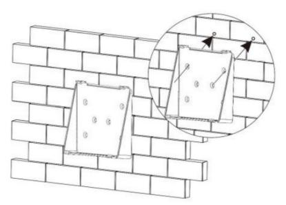
Match the bracket's upper buckle with the DTU-Pro/DTU-Pro-C.
