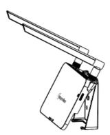
Match the bracket's lower buckle by gently pressing the lower side of the DTU-Pro/DTU-Pro-C until
