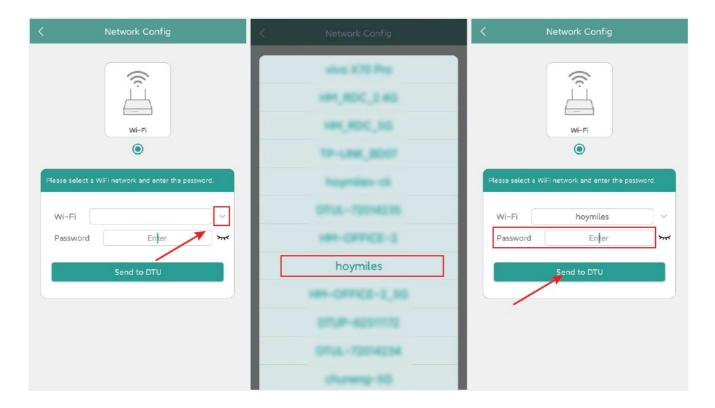
Select the router Wi-Fi and enter the password. Click "Send to DTU".
