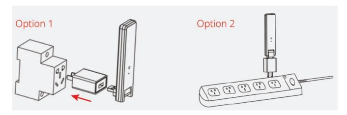
Option 2: Connect the DTU to the adapter and plug it into the power strip.
