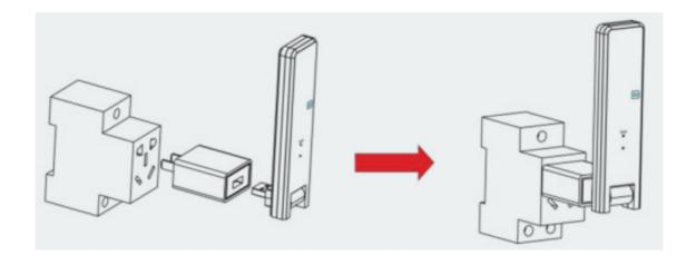
**Option 2:** Connect the DTU to the adapter and plug it into the power strip. Please make sure that it is placed at least 0.5 meters above the ground, and try to install the DTU at a 90 degrees angle perpendicular to the ground.
