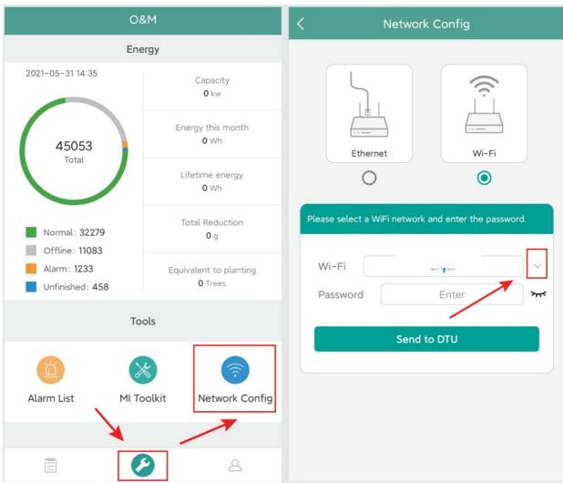
– Use a LAN cable, with one end connected to the house router and the other to the DTU Ethernet port. Use the smartphone/tablet to open the Installer App and login. Locate "O&M" on the bottom of the page, select "Network Config", and then select "Ethernet" (if Ethernet option is selected).
