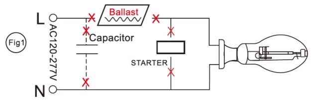
2. Connect Supply Line and Neutral directly to the existing lamp holder. Shown as Figure 2
