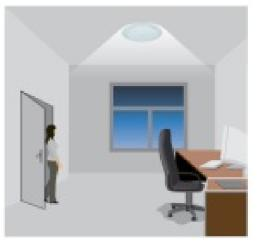
With insufficient natural light, the sensor switches on the light automatically when presence is detected. After hold-time, the light dims to stand-by level if the surrounding natural light is below the daylight threshold.
