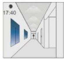
When the natural light level exceeds setpoint off to light, the light will turn off even if when the space is occupied. The light automatically turns on at 10% when natural light is insufficient (no motion).
