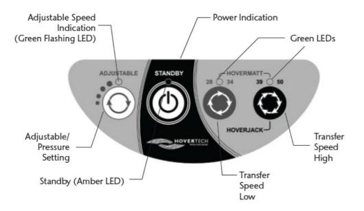
ADJUSTABLE: For use with HoverTech air-assisted positioning devices. There are four different settings. Each press of the button increases the air pressure and rate of inflation. The Green Flashing LED will indicate the inflation speed by the number of flashes (i.e. two flashes equals the second inflation speed).
