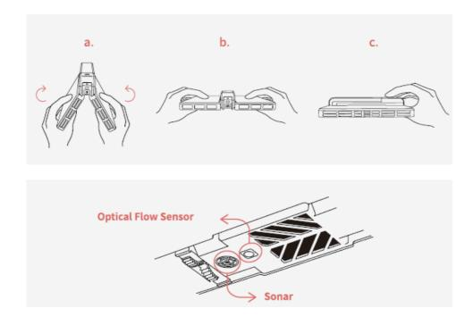
Caution: Do not cover the optical flow sensor or sonar before releasing it.
