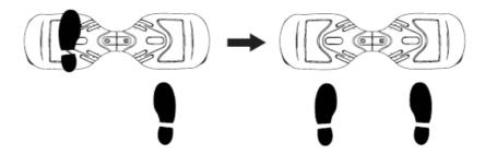
**WARNING** Make sure to lift your feet completely off the foot mat to clear the Maverick when stepping back to dismount. Failure to do so may send the Maverick into a tailspin.
