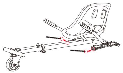
3. Wrap the straps underneath the hoverboard and pull them through to the other side. Insert the straps into the rear hole of the handlebar mounts. Fasten the front and rear sides of the straps. Make sure they are tightly secured to the hoverboard.
