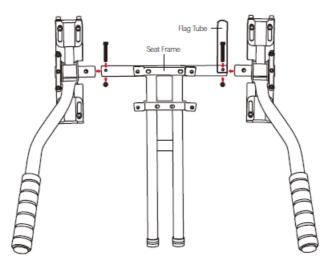
3. Insert the front frame into the seat frame. Adjust the front frame to your preferred length. Remove the black bolt and the °irst white washer from the end of each locker. Fully insert the screwed section of one locker into the seat frame holes. Add the white washer and black bolt back onto the locker once it is fully inserted and twist them on clockwise until they are tightly secured. Close the locker clamp tightly. Repeat these steps on the other side of the seat frame with the other locker.
