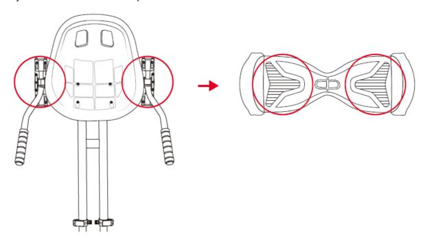
2. Secure your Hover-1 Kart to your hoverboard using 2 of the included hook and loop straps. With the fastener side facing away from your hoverboard, thread the straps through the outside hole of each handlebar mount.
