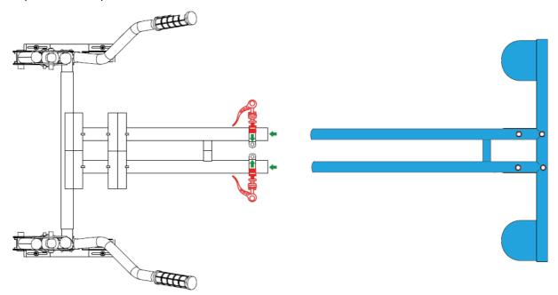
4. Align the holes of the seat with the holes of the seat frame as show below. Insert the M6 X16 screws. Attach the 20 mm washers and the 6 mm nuts to the bottom of each screw, under the seat frame. Twist the nuts on clockwise. Hold the 6 mm nuts still with the wrench while turning the screws clockwise with the larger hex key to tighten the screws. Make sure all 4 screws are tightly secured.
