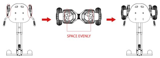
2. Secure the Beast Buggy to your hoverboard using 2 of the included hook and loop straps. The other 2 straps included are spares. With the fastener side facing away from your hoverboard, thread the straps through the front hole of each handlebar mount.
