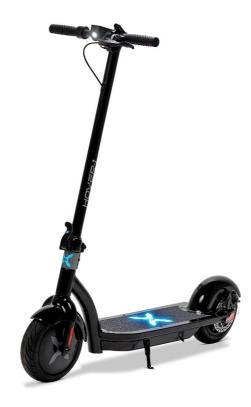
As with all mechanical components, the Hover-1 Alpha is subjected to wear and high stresses. Different materials and components may react to wear or fatigue in different ways. If the design life of a component has been exceeded, it may suddenly fail possibly causing injuries to the rider. Any form of crack, scratch, or change of coloring in highly stressed areas indicates that the life of the component has been reached and it should be replaced. Do not ride in an abusive manner.
