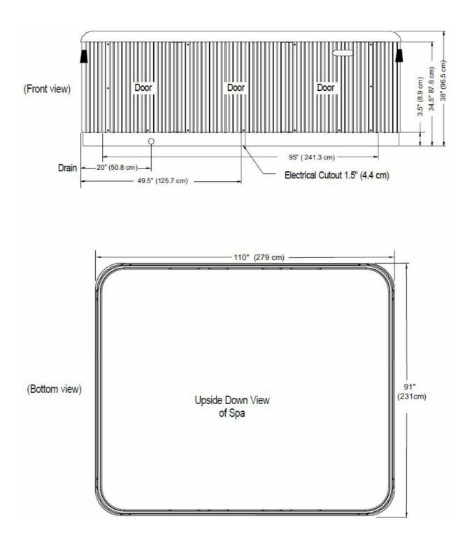
Watkins Manufacturing Corporation recommends that the Gleam be installed on a minimum 4" (10 cm) thick reinforced concrete pad or structurally sound deck able to support the "dead weight" found in the spa specification chart.
