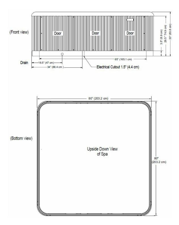
Watkins Manufacturing Corporation recommends that the Bolt be installed on a minimum 4" (10 cm) thick reinforced concrete pad or structurally sound deck able to support the "dead weight" found in the spa specification chart.
