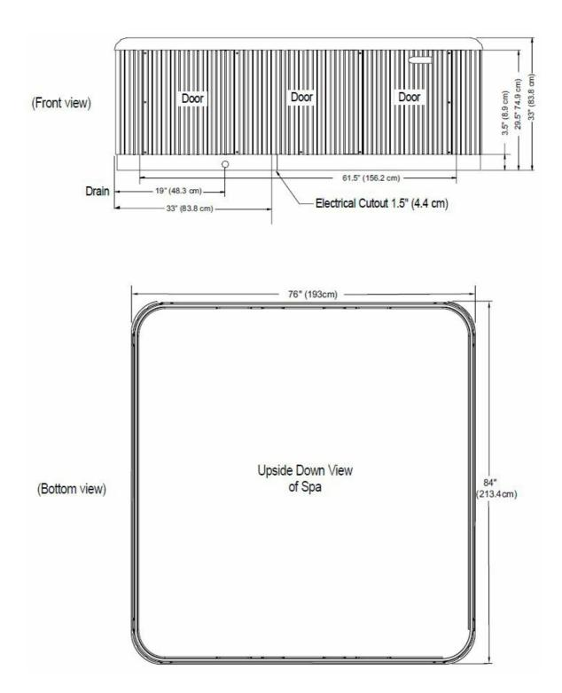
Watkins Manufacturing Corporation recommends that the Glow be installed on a minimum 4" (10 cm) thick reinforced concrete pad or structurally sound deck able to support the "dead weight" found in the spa specification chart.
