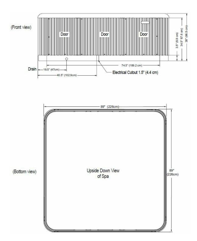
Watkins Manufacturing Corporation recommends that the Pulse be installed on a minimum 4" (10 cm) thick reinforced concrete pad or structurally sound deck able to support the "dead weight" found in the spa specification chart.
