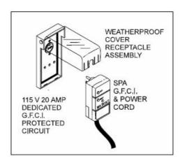
The Ground Fault Circuit Interrupter (GFCI) is located at the end of the power cord. This device is for your protection. It is very important to protect it from rain and other moisture. Test once a month, with the plug connected to the power supply,
