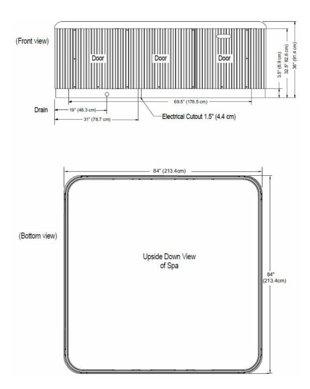
Watkins Manufacturing Corporation recommends that the Flair be installed on a minimum 4" (10 cm) thick reinforced concrete pad or structurally sound deck able to support the "dead weight" found in the spa specification chart.
