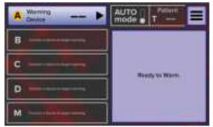
Plug in a Warming Device to begin. When the cable is properly inserted into the Controller, an audible sound indicates that the Device is properly connected, and its port icon illuminates on the screen.
