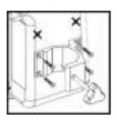
Line up the mounting clamp with the bottom two sets of screw holes.
