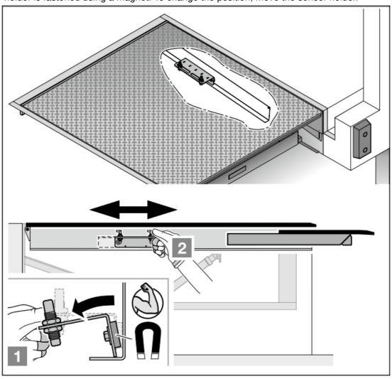
Reposition the sensor holder. Measure the distance from the inside of the rear rail of the platform.
