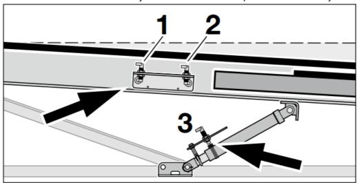
The sensor holder for sensor 1 and 2 must be at the bottom of the platform beam. Sensor 3 must be able to detect the bolt of the hose clamp.
