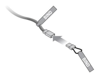
The receiver must be bound to your transmitter before it will operate. Binding is the process of teaching the receiver the specific code of the transmitter so it will only connect to that specific transmitter.
