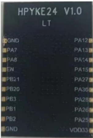
Figure 3. Pin definition (Bottom view)
