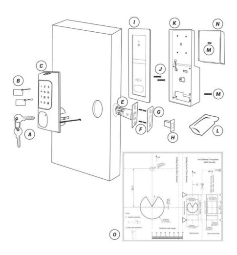
**NOTE:** SCREWS FOR DOORS WITH A THICKNESS OF 35 TO 55 MM ARE INCLUDED IN THE STANDARD PACKAGE.
