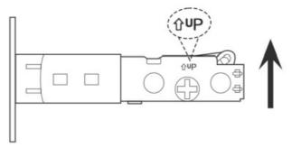
Insert the latch and ensure it is parallel to the door face.
