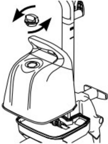
2. Align the tank and firmly press it into place.
