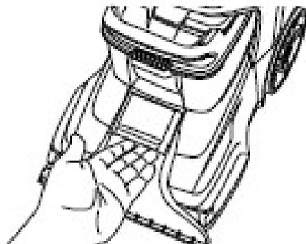
2. Hold open the Hose Solution Port door. Plug the Hose Solution Tube connector firmly into the Hose Solution Port.
