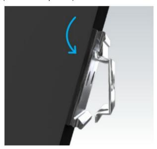
2. Now press the gateway straight down. Make sure not to release it until it has clicked into the lower fixture.
