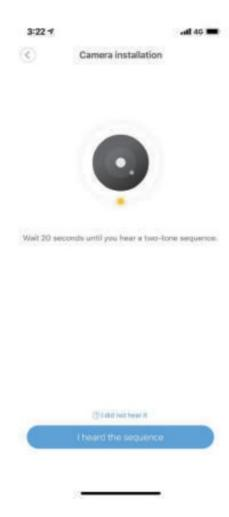
If you don't hear the sequence, please press the "RESET" on the device. Continue for more than 5 seconds, until you heard the sequence, that means the reset is successful.
