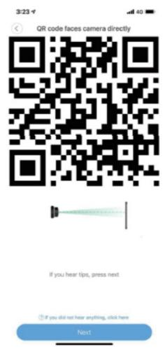
The QR code that appears on the mobile phone is scanned against the camera lens, and the device emits a prompt sound "QR code scan successful" and "WiFi connected", click Next, and wait for the network configuration to be completed.
