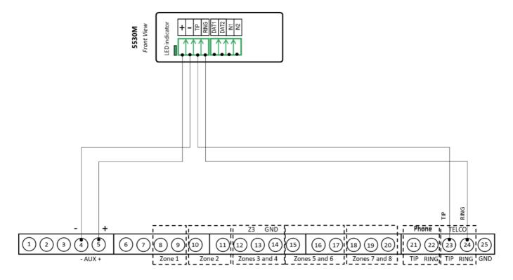
Wiring and Programming Uplink Communicators to Honeywell Vista 20SE
