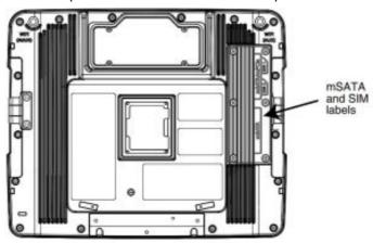
5. Remove the access panel from the opening and press the UPS battery disconnect button located between the primary mSATA drive and the SIM card/secondary mSATA installation slots.
