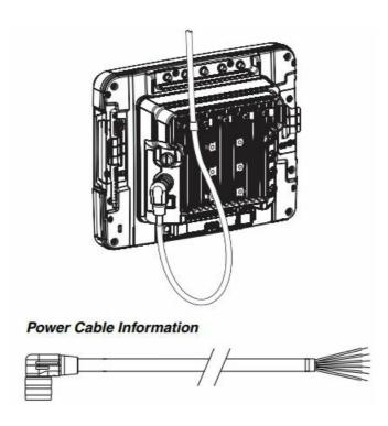
Twist the red and red/white wires together and twist the black and black/white wires together before connecting to vehicle power. Connect the green wire to the vehicle ground:
