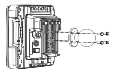
3. Attach VM1A assembly to RAM base using RAM arm and tighten knob on RAM arm.
