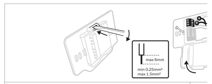
A) Separate the wallplate from the thermostat, and using a screwdriver open the wallplate terminal cover to connect wires.
