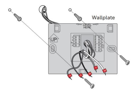
**Note**: You may be able to use your existing wall anchors. Hold the wallplate up to the existing anchors to check for alignment.
