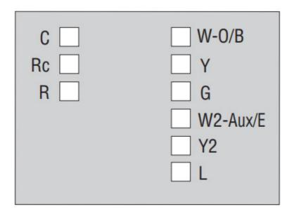
Note: The L terminal on the lower right is used only for Heat Pump systems.
