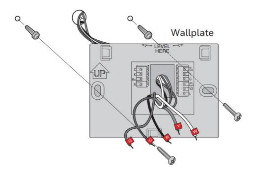
**Note**: You may be able to use your existing wall anchors. Hold the wallplate up to the existing anchors to check for alignment.
