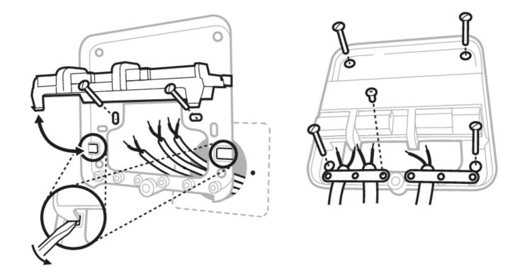
Attach the new cover and turn the power on
